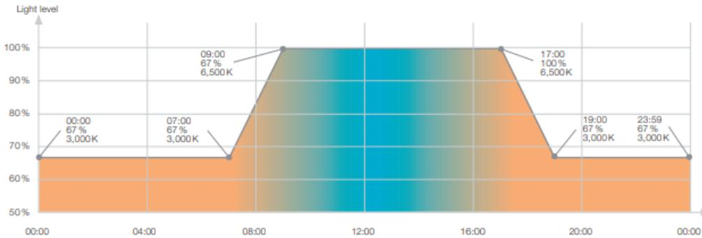
HCL will start automatically with default settings after synchronizing the real-time clock. Automatic sync done by connecting with the DALI CONFIG APP.
