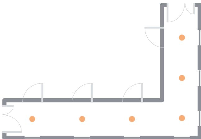
The lights will be switched on automatically when a person enters the corridor and automatically dimmed down to a light level of 10 % after the delay time has expired and if no presence is detected.
