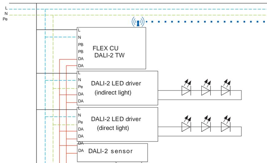
d) Wiring diagram of zone 5 with standard DALI luminaires
