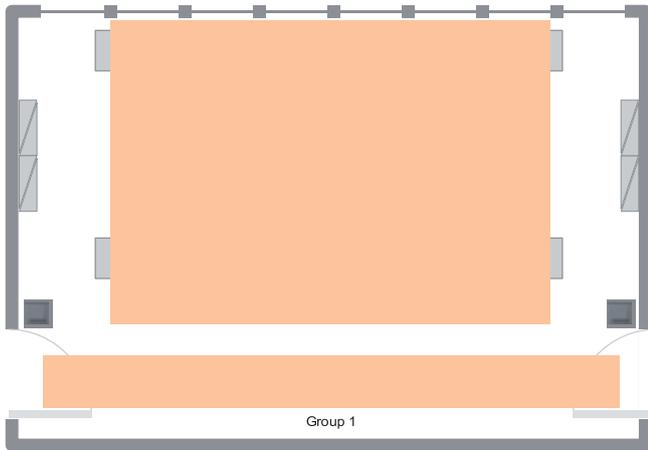
The open-plan office luminaires are floor-standing luminaires in the desk area and downlights in the corridor area. The desk luminaires are wirelessly interconnected and react as a big swarm as soon as presence is detected by one of the Swarm luminaires.
