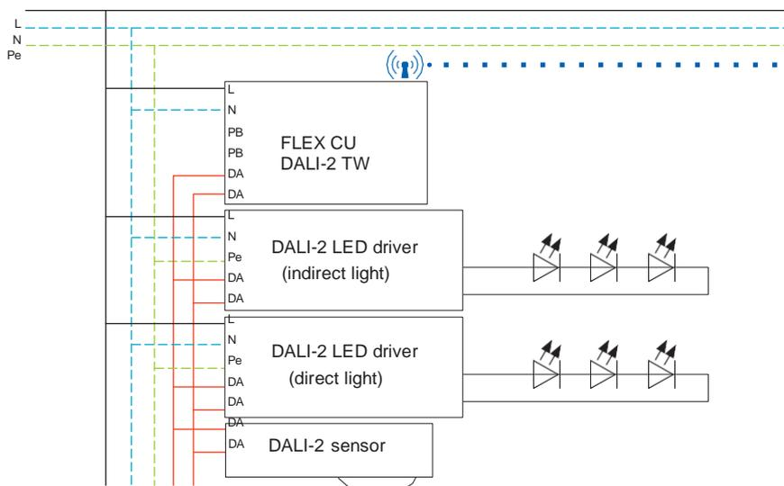
b) Wiring diagram of group 1 with standard DALI luminaires
